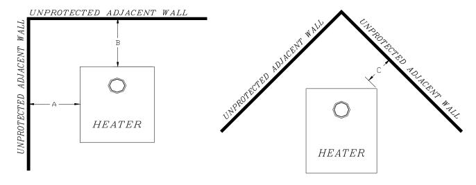
FIGURE 1.3 Clearances to combustible materials
